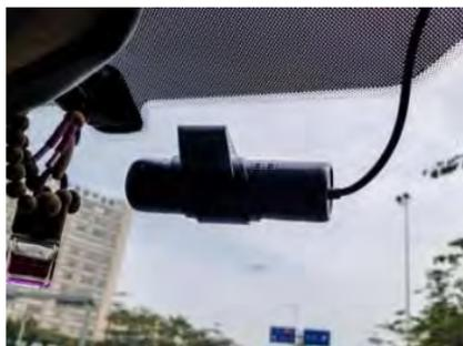
5. Route the power cable by tucking it neatly across the top of the windscreen and down the A pillar. This is located at the side of the windscreen, down the same side of the vehicle where the fusebox is located.
