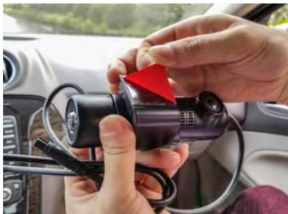
1. Firstly, decide the optimum position for the unit, ensuring that it does not obscure the driver's view. The best position is usually in the center of the windscreen at the top,
