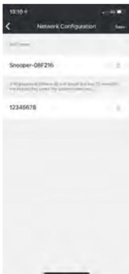
The network configuration interface is used to modify the WiFi name (SSID) and password.
