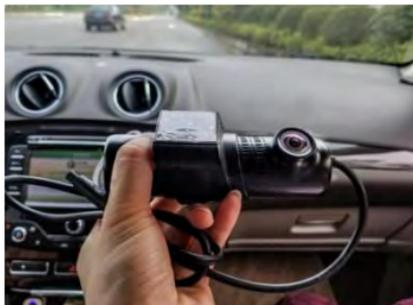
2. Secondly, clean the area of the windscreen where the unit is to be fitted.
