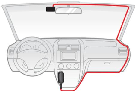
3. When adjusting the angle of mounting, make sure that the camera's view is parallel with the level ground and the ground/sky ratio is close to a 50/50 split.
